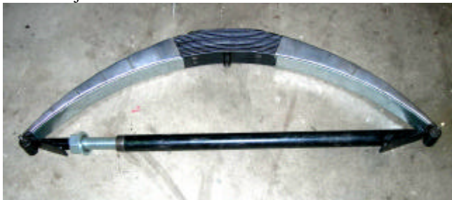
This spring spreader will handle any job! Made by Clift Harden, modified by Dubois and Gunnarson.
